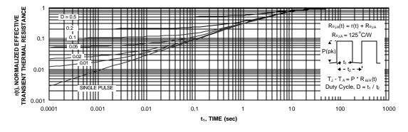
Figure 11. Transient Thermal Response Curve.
