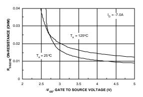
Figure 4. On-Resistance Variation with Gate-to-Source Voltage.
