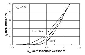
Figure 5. Transfer Characteristics.
