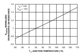
Figure 3. On-Resistance Variation with Temperature.
